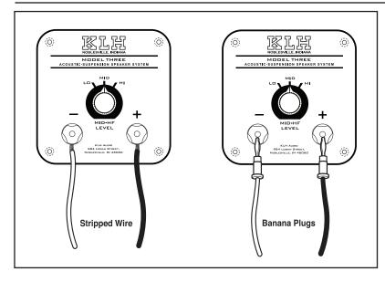
IMPORTANT! Turn your amplifier or receiver OFF before connecting your speakers. This action will avoid damage that could result from accidental shorting of the speaker cables.
